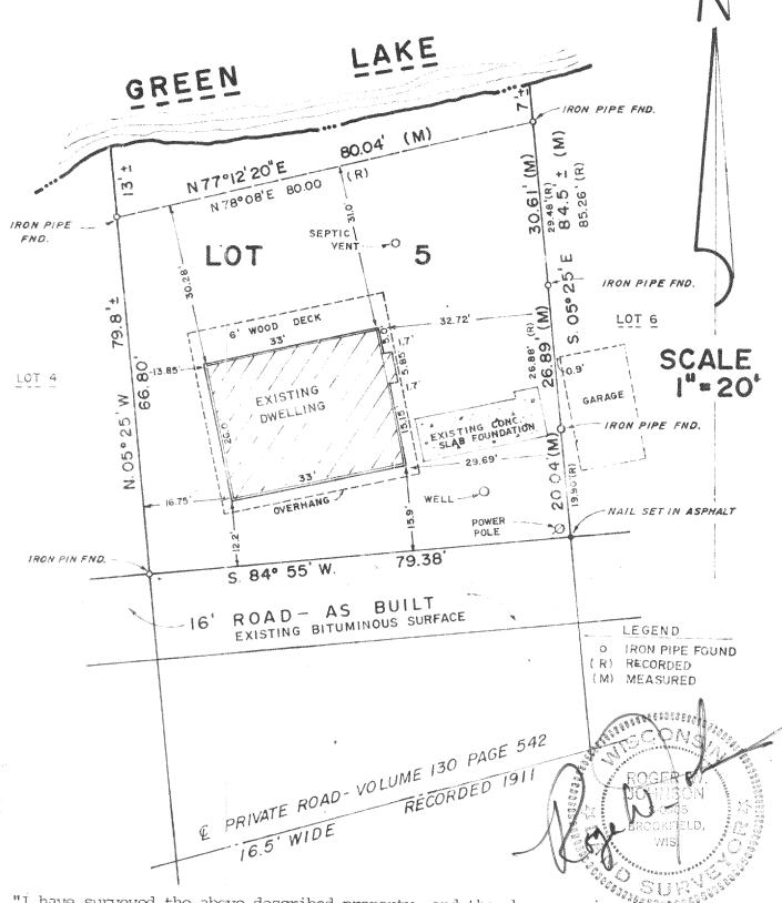
"I have surveyed the above described property, and the above map is a true representation thereof and shows the size and location of the property, its exterior boundaries, the location and dimensions of all structures thereon, fences, apparent easements, roadways and visible encroachments.
